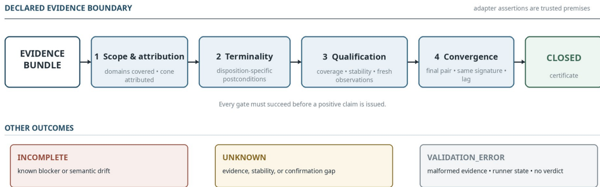
Figure 2. BAC decision path for a validated evidence bundle. A positive certificate requires every gate. Known blockers or final semantic drift yield INCOMPLETE ; evidence, stability, or confirmation gaps yield UNKNOWN . Malformed evidence terminates as VALIDATION_ERROR before verdict evaluation. Adapter assertions remain trusted premises under declared source contracts.
